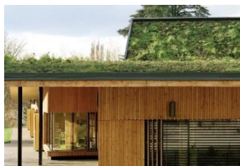
Toiture intensive (substrat 12 cm)
